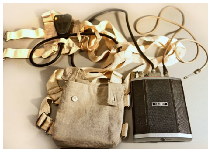
Complete Kaira with associated linen body harness for carrying the set under the clothes on the chest.
