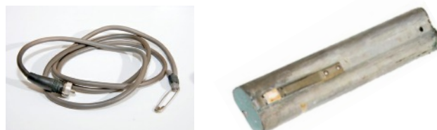
Flexible wire aerial with safety pin for attaching to the clothes. (Left) The battery/rechargeable accumulator holder was identical to that of the Chaika. (Right)
